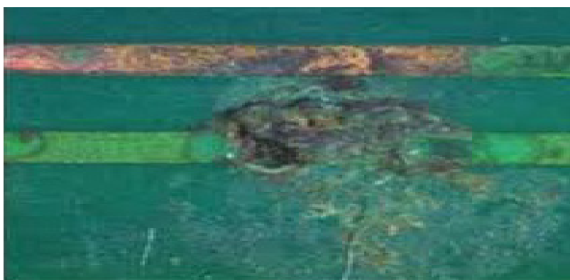
Conductors corrosion on PCB (photo by EDN)
